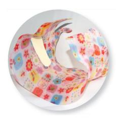
The material **Lunatec motion** can also be used for general orthopaedics, prosthetics and orthotics, e.g. as cushioning in classical orthopaedic devices or as a functional lining on support orthoses and corsets. Besides its excellent **damping** and **pressure spread**, it also has a **good absorption of shearing forces**, making it ideal for pressure sensitive areas exposed to forces from body movements.
